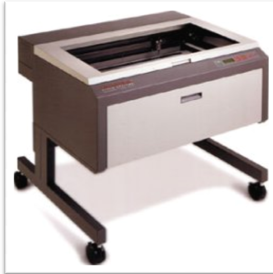
Figure 7. CNC LASER milling machine. Used in all milling operations for the LTCC micro combustor (Systems, Universal LASER, 2009).
