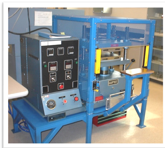
Figure 9. Laboratory unidirectional hot press. Used for prelamination of LTCC layers (Plumlee, 2007).
